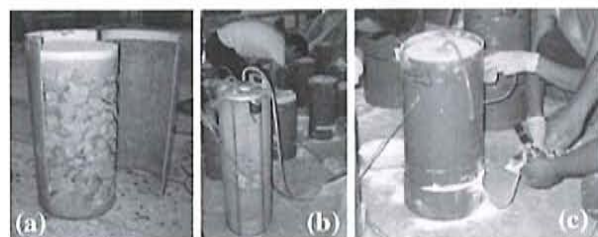
Fig. 2 a UngROUTED cylinder, b and c injecting the cylinders
