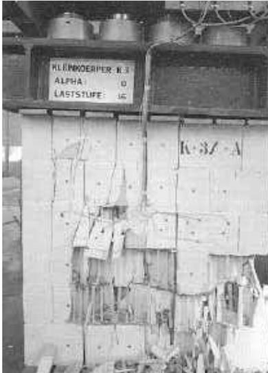
a) Compressive failure of units
