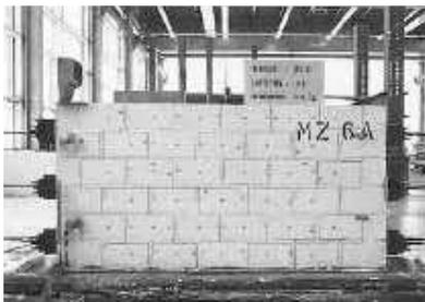
d) Tensile failure along joints
