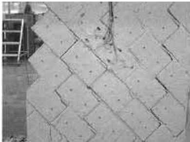
b) Sliding failure along joints
